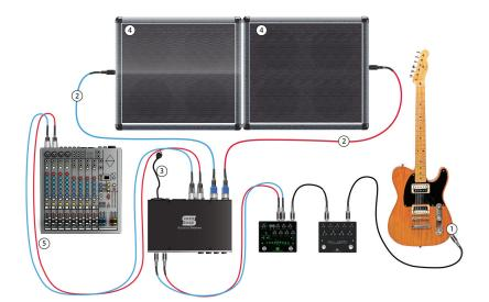
Use high quality **speaker cable(s)** [2] to connect your PowerStage 700's **Speaker Output jack(s)** to the input of a **4 - 16 ohm cabinet** [4] or cabinets. PowerStage 700 uses Neutrik combi-jacks for compatibility with both speakON and quarter-inch speaker cables. Using the supplied **power cable** [3], connect the PowerStage 700 to a power outlet.
